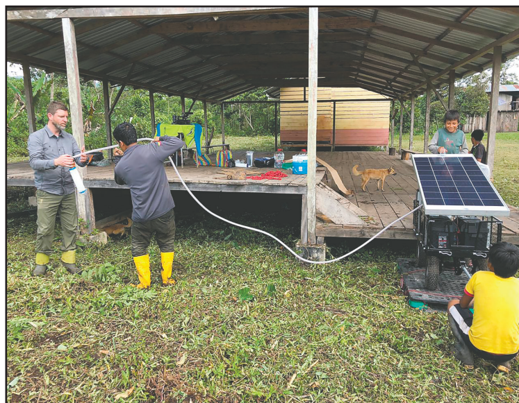
A mobile, solar-powered water purifier in action.
